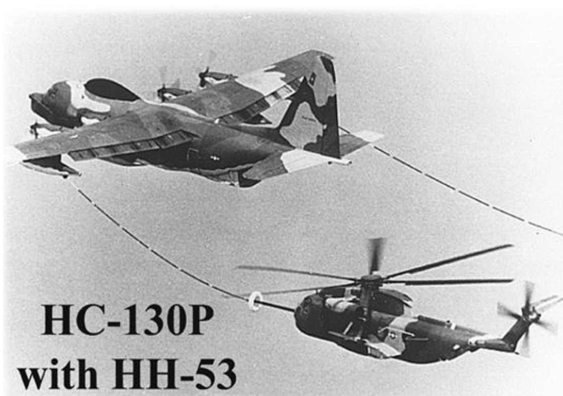
HC-130P tankers (Lime One and Two) provided refueling for the raid's helicopters.
